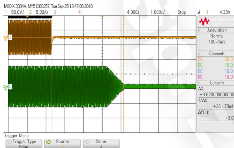
Figure 3: Fail-safe test on 1.2kW single phase system
