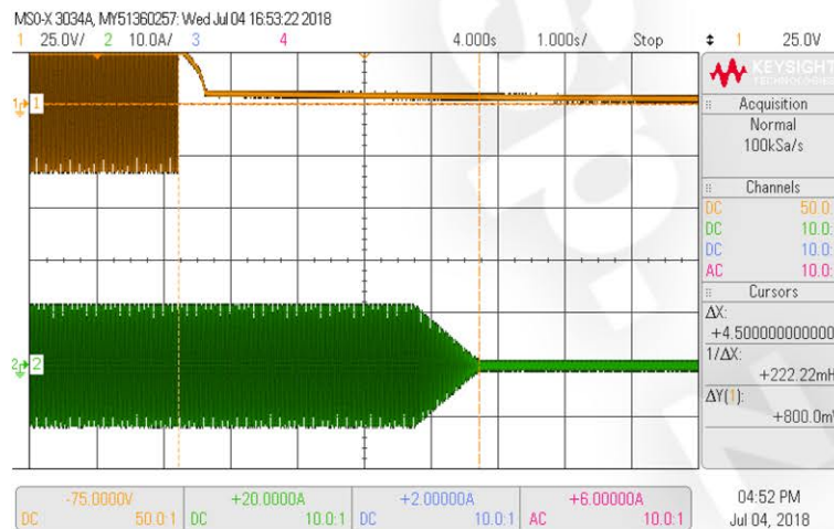
Figure 6: Fail-safe test on 1.8kW single phase system
